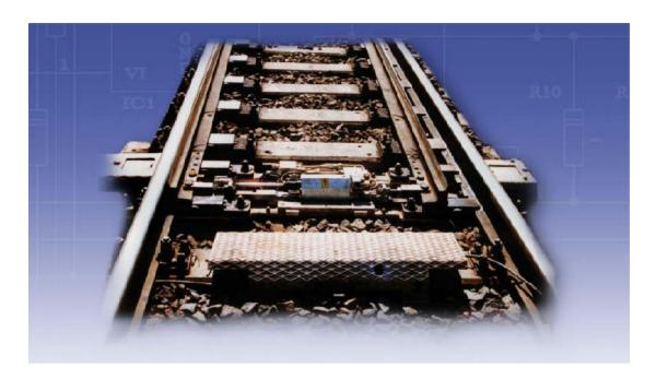
MA-HVH type point-setting machine serves for setting the point rails of the railway turnouts by electrically-operated hydraulic energy, their hydraulic and mechanical locking, checking their end-positions and checkback in an electrical way. The point setting mechanism is suitable for simultaneous synchronized setting of both simple and high radius turnouts, fixing the different lock assemblies, checking of end-positions and also suitable for check-back.
